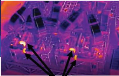
Heat Loss, shows signs of metal fatigue.
